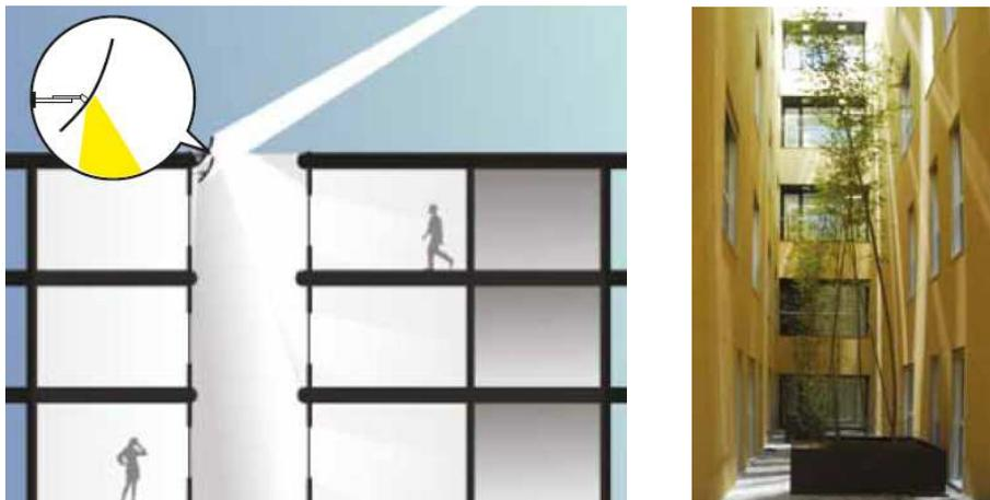
Figure 17: Graphic scheme of the effect of reflectors in an atria (left). On the right, a real case (extracted from Deplosun – Espacio Solar brochure).
