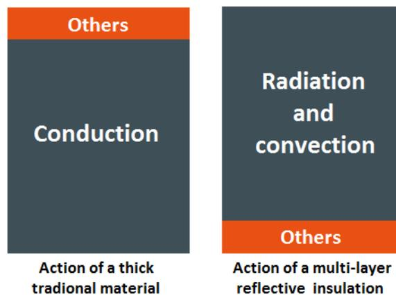
Figure 6: Different effects of conventional materials: EPS, XPS, mineral wool... (left) and MLI (right).
