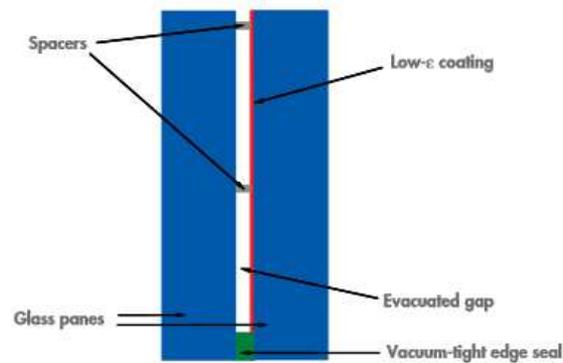
Figure 10: Composition of vacuum glazing.
