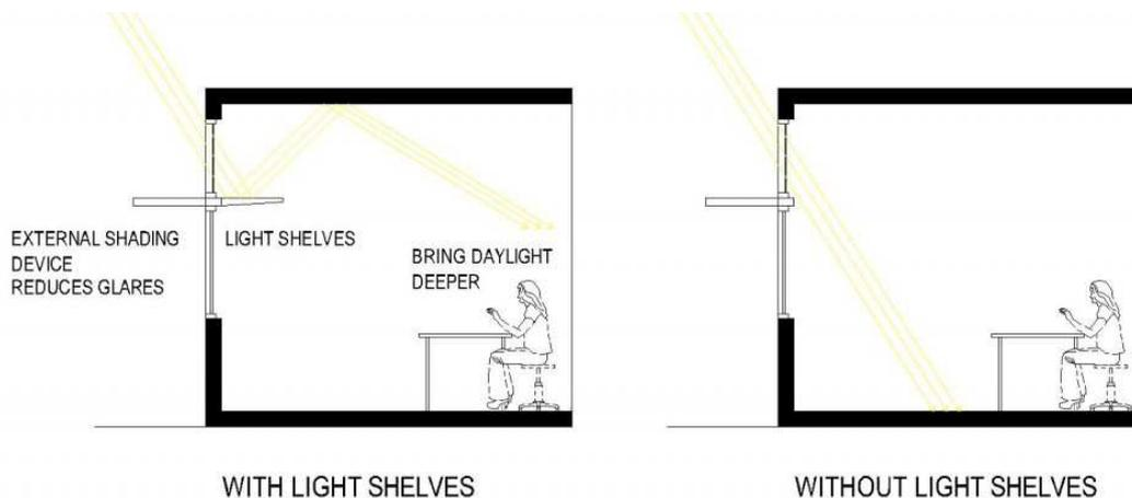
Figure 23: External Shading devices with light shelves (left) and without them (right). Courtesy of [www.greenasiaforce.com](http://www.greenasiaforce.com)
