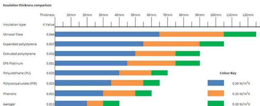
Figure 2: Insulation thickness comparison for different targeted U-values<sup>5</sup>
