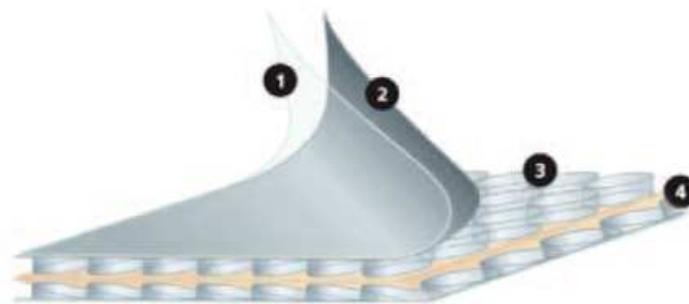
Figure 5: Reflectix multi-layer sheet composition. 1- Anticorrosive layer. 2- Aluminium layer. 3- Bubble wrap. 4- Polyurethane foam.
