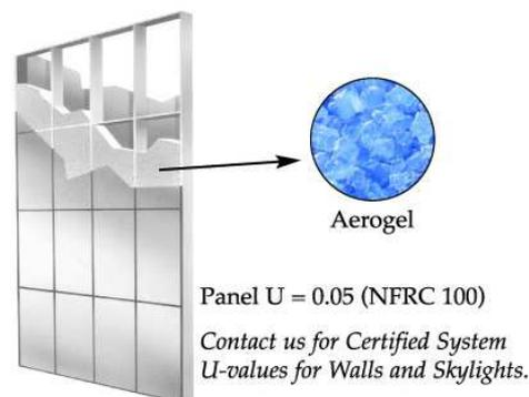
Figure 11: Sketch of a panel filled with granular aerogel. Courtesy of [www.kallwall.com](http://www.kallwall.com)
