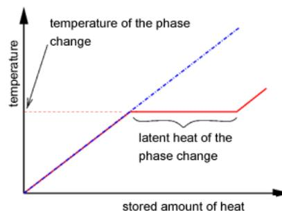
Figure 24: Comparison of the storage processes for sensible (blue) and latent (red) heat.
