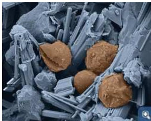
Figure 25: PCM in gypsum plaster. BASF.
