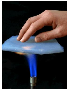
Figure 3: A demonstration of aerogel's insulating properties.
