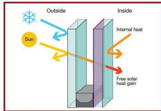
Figure 9: Brief summary of the effect of low-e glasses. Courtesy of [www.glassforeurope.com](http://www.glassforeurope.com).
